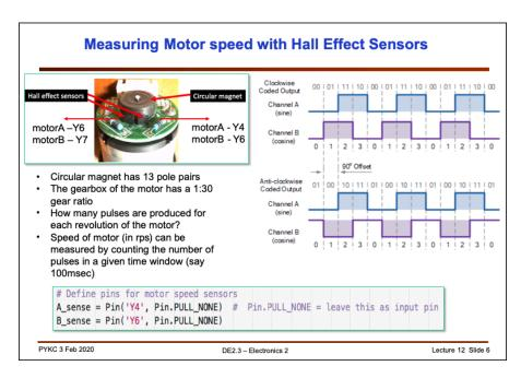
Next, we use the Hall Effect Sensors (two) on the motor to determine the speed of the motor and direction of the motor. The questions to ask yourself are:
