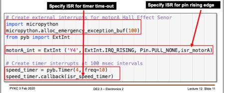
How does one set up interrupts in MicroPython using the Pyboard and the Pybench System? First you need to include the following statement to allocate memory to store the state of the program:
