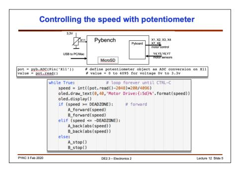
Next, we use the potentiometer (5k $\Omega$ ) to control motor speed and direction. Here are the questions to test yourself:
